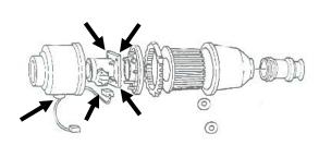
7. Using a 10mm socket, remove the four MAF sensor mounting nuts. Carefully remove the MAF sensor and the wiring harness from the airbox, (save them for reuse).
