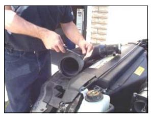
**4.** ) Remove the factory intake tube, and set it aside. Remove the **AIT** sensor from the tube by carefully prying it out with a flat blade screwdriver (save the sensor for reuse). Disconnect the **Mass Air Flow** (**MAF**) sensor wiring harness from the main engine wiring harness.
