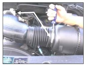
**2.** Loosen the hose clamps at the throttle body, and air filter housing outlet.
