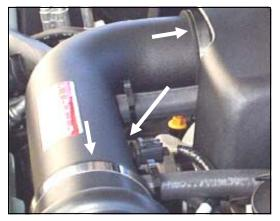
11. Install the 7/16" rubber grommet (#15) into the Airaid Intake Tube (#2). Insert the factory AIT sensor into the grommet. Slip the Airaid Intake Tube into the urethane hump and reducer hoses. Align for best fit and tighten the remaining hose clamps. Tighten the MAF bracket and reconnect the AIT sensor wiring harness.
