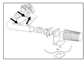
**15.** <u>4.6L engines continued</u>: Connect the Airaid Intake Tube nipple to the IABV inlet tube using the  $3/4 \times 1/2$ " L-hose (#7), and two #22 speed clamps (#17).
