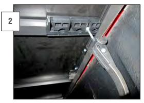
Refold the tonneau cover, without moving it side to side and connect the front latches. Insert the latches into the first hole, then back over the hump. Hold the handle horizontally, place the clamp under the bed lip and push the handle to a vertical position. If the handle is not tight enough it can be loosened, then rotated to the right to tighten the clamp and hold the cover securely. Repeat the same procedure with the rear (2) clamps.
