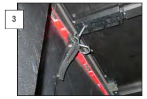
Make sure the clamp is secured to the metal bed lip and not just the plastic. If the clamp does not sit securely on the metal the plastic can be trimmed.
