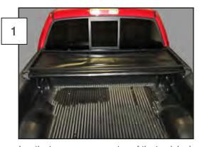
Lay the tonneau cover on top of the truck bed sides. Align the front of the cover with the front of the bed. Be sure that the plastic clips holding the cover are facing upward and accessible. Unhook the plastic clips and unfold the tonneau cover. Align the tonneau cover on the truck.
