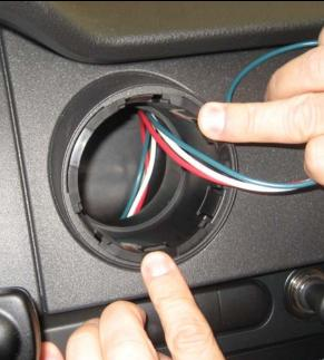
8. Feed the wiring through the VentPod and install the VentPod into the inner vent structure (see note below).
