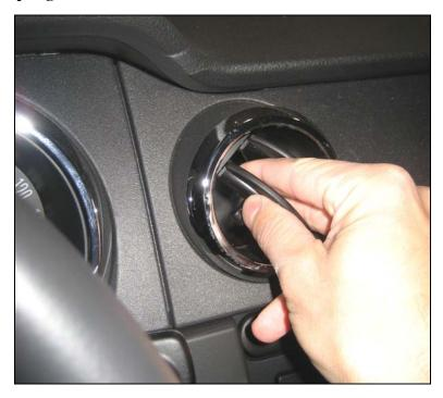
2. The VentPod will reuse the factory trim ring/bezel which is secured to the stock vent with four locking tabs (only two locking tabs for F150 customers). To remove the bezel, **CAREFULLY** wedge a small, flat head screwdriver between the base and bezel locking tabs.
