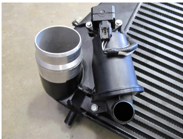
Fig. 1-r (Vortech cooler w/ bypass valve assembly)
