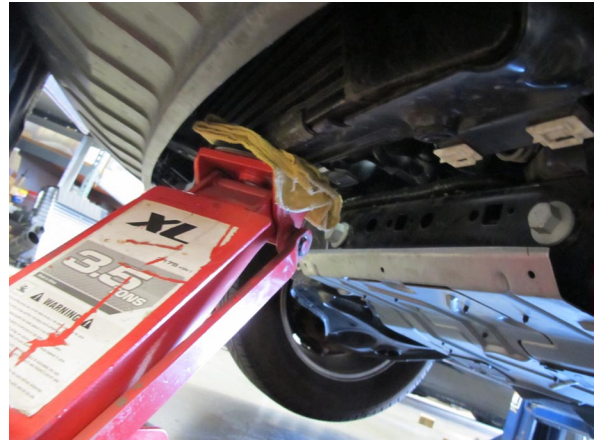
Fig. 2-a (Position cooler from underneath)
