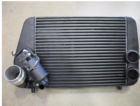
Fig. 1-q (Vortech cooler w/ bypass valve assembly)
