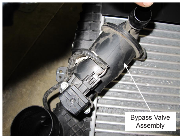
Fig. 1-p (Turn counter-clockwise to release)
