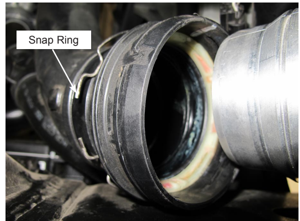
Fig. 1-f (Release snap ring & pull away)
