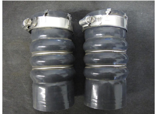
Fig. 1-e (Discard OEM couplers & hose clamps)
