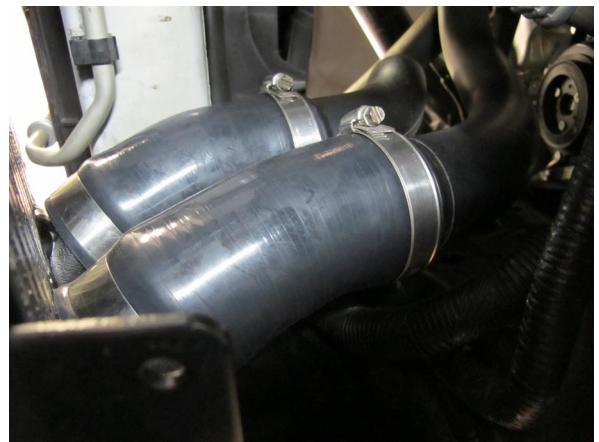
Fig. 2-h (Installed couplers & hose clamps)
