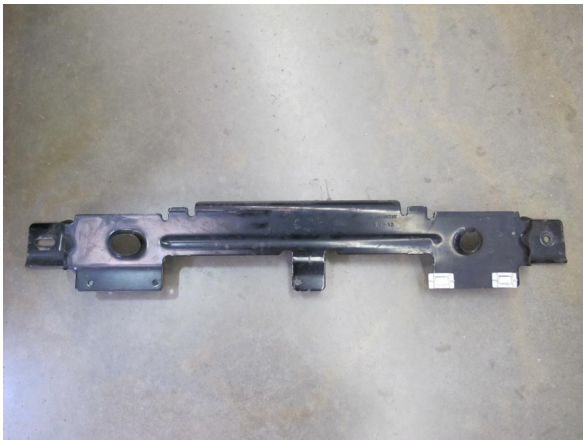
Fig. 1-k (Lower cooler support bracket)
