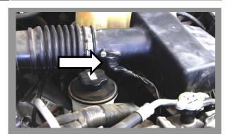
Disconnect the Mass Air Flow (MAF) Sensor.
