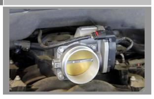
Bolt on the BBK Throttle Body and reconnect the connector.
