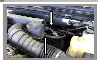
Remove the two vent hoses going into the factory intake system.
