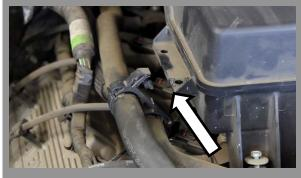
Loosen the two 10mm mounting bolts that secure the factory intake system to the vehicle. Also remove the clip on the passenger side of the stock intake system using pliers.
