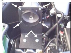
**8.** Mount the **MAF** sensor to the MAF bracket (#3) using four 1/4-20x 7/8" hex bolts (#8), 1/4-20" nylock nuts (#10), and the MAF gasket (#11). Mount the bracket and sensor to the factory location, using the MAF backing plate (#12), two 1/4-20x 7/8" hex bolts (#8), four 1/4" flat washers (#9), and two 1/4-20" nylock nuts (#10). (Leave the MAF bracket loose for now).
