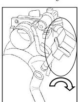
**14.** <u>4.6L engines</u>: Rotate the *LABV* inlet tube 90 degrees to provide clearance for the 3/4 x 12" L-hose (#7).
