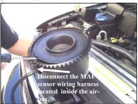
**6.** Locate the notch on the flat side of the airbox and gently pry it up. Disconnect the **MAF** sensor wiring harness from the sensor (inside the airbox).
