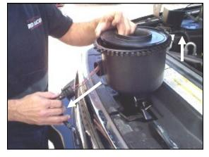
**5.** The factory airbox assembly is held in place by rubber grommets (it is a "pull to release fit."). Remove the assembly and grommets from the engine compartment. Unlatch the airbox and separate the two sections. Remove the wire loom from the **MAF** sensor wiring harness, then slide the grommet away from the connector.
