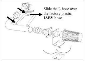
**13.** <u>5.4L engines</u>: Measure and cut the 3/4 x 12" L-hose (#7) as needed, then slide it over the factory plastic **IABV** hose. Install the hose onto the Airaid Intake Tube nipple and secure it using two #22 speed clamps (#17).
