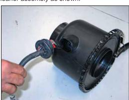
16. Slide the rubber grommet back to gain access to the mass air sensor electrical connector. Using a small screw driver, release the red locking tab and disconnect the electrical connection and remove the wiring harness.
