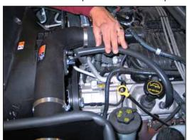
27. Install the supplied crankcase vent hose onto the valve cover and secure with the provided hose clamp then connect the other end onto the intake tube as shown.
