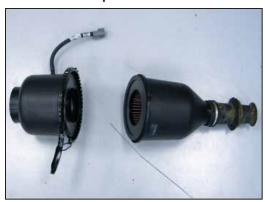
15. Release the clam shell clamp to open the air cleaner assembly as shown.
