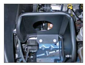
13. Install the heat shield assembly into position with the rubber insert nuts installed into the small portion of the factory holes.
