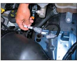
5. Unhook the secondary mass air sensor connection from the clip which holds it to the airbox mounting bracket, and then disconnect the secondary mass air connection.
