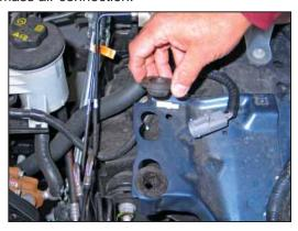
6. Remove the two airbox mounting grommets from the bracket as shown.
