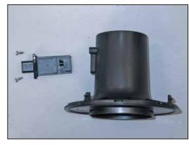
18. Using the supplied T20 TORX, remove the two screws which secure the mass air sensor and remove the mass air sensor as shown.
