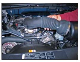
3. Loosen the hose clamps which secure the stock intake tube to the throttle body and air filter housing and then remove the intake tube from the vehicle.
