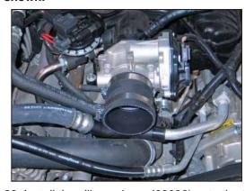
22. Install the silicone hose (08096) onto the throttle body and secure with the provided hose clamp.
