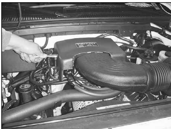
2. Loosen and remove the three bolts that retain the throttle body cover, then remove the cover.
