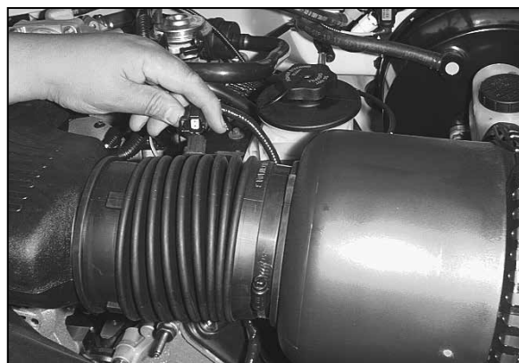
3. Disconnect the air temperature sensor electrical connection.
