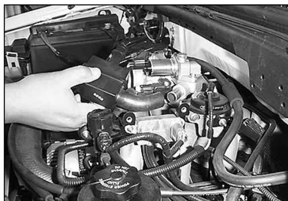
4a. On models with 4.6L engines, detach the air bypass valve and crankcase vent hose from the stock intake tube.
