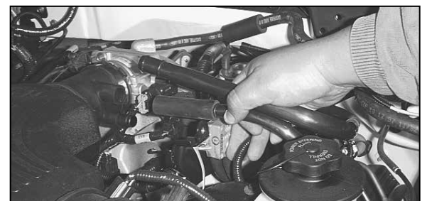
4b. On models with 5.4L, detach the idle air control and crankcase vent hose from the stock intake tube.
