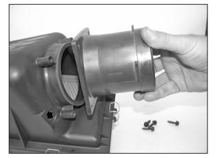
25. Remove the mass air sensor from the factory air box as shown.
