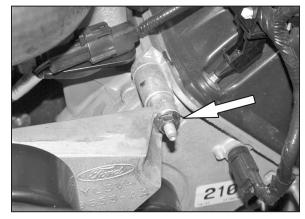
13. Remove the 8mm nut from stud that retains the idler pully bracket.
