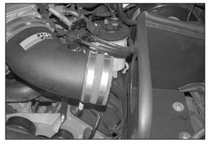
27. Install the silicone hose (08761) onto the intake tube with the provided hose clamps.
