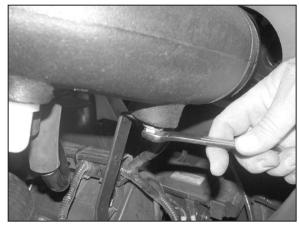
22. Connect the new intake tube to the bracket with the provided hardware as shown.
