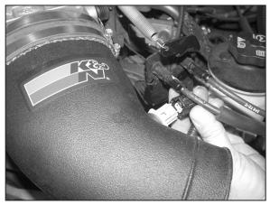
24. Install the temp sensor into the intake tube then reconnect the electrical connection as shown.
