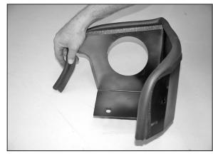
9. Install edge trim onto the heat shield as shown. Trim if needed.
