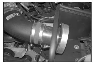
28. Install the mass air sensor assembly onto the intake tube, then secure with the provided hose clamp.
