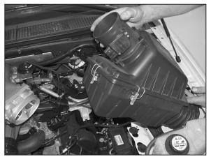
6. Pull up firmly on the factory air box to remove from vehicle.
