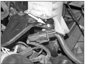
4. Unhook the secondary mass air sensor electrical connection from the power steering reservoir bracket, then unlock the electrical connection locking tabs and separate the electrical connection
