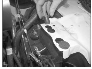
8. Install the provided nut inserts into the air box mounting holes as shown.
