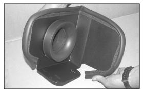
15. Install the provided edge trim onto the heat shield as shown.
