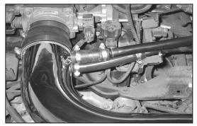
25. On V8-5.4L models slide the provided 5" long silicone hose onto the hard line, then trim hose for best fit before connecting to the vent on the K&N<sup>®</sup> intake tube as shown.
