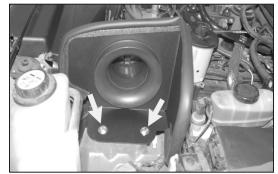
17. Install the heat shield assembly into the vehicle and secure it to the stock air cleaner grommets using the provided hardware but do not tighten completely at this time.
