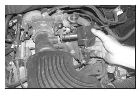
4. On 4.6L equipped vehicles, remove the idle air control hose and chamber as shown. Then, disconnect the crankcase vent hose from the factory intake tube.
