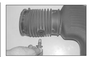
7. Remove the air temperature sensor from the stock intake tube as shown.
