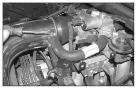
24. On vehicles equipped with a 4.6L engine, attach the provided 5/8"id idle air by-pass vent hose onto the appropriate fitting on the K&N<sup>®</sup> intake tube, trim for proper fitment to prevent the hose from developing a kink and attach the open end to the idle air by-pass valve.
