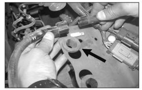
9. Unclip the mass air sensor wire harness from the air cleaner tray, then, disconnect the secondary mass air sensor electrical connection and remove the air cleaner assembly.
