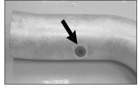
19. Install the provided rubber grommet into the hole on the  $K\&N^{\textcircled{B}}$  intake tube as shown.
