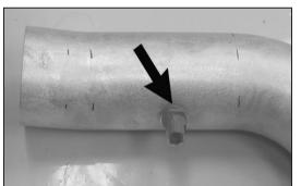
20. Install the air temperature sensor from step 8 into the rubber grommet as shown.
