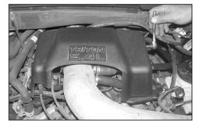
27. Re-install the engine cover and secure with the stock bolts.
