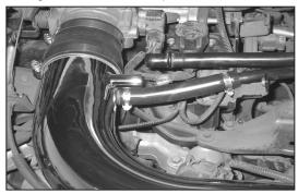
23. Install the provided  $5/8^{\circ}$  silicone hose onto the stock plastic crankcase vent line. Then, install the open end of the  $5/8^{\circ}$  ID silicone hose onto the K&N<sup>®</sup> intake tube and secure with the provided hose clamps.
