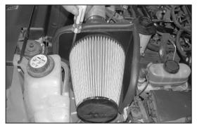
30. Install the K&N $^{\mbox{\tiny B}}$  air filter and secure with the provided hose clamp as shown.
