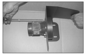
14. Bolt the stock mass air sensor onto the provided heat shield using the provided mass air adapter, gaskets and the provided hardware as shown.
