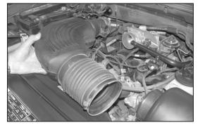
6. Loosen the hose clamps at the throttle body and at the air cleaner, then, remove the stock intake tube as shown.
