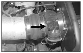
29. Reconnect the primary mass air sensor electrical connection as shown.
