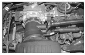
3. On vehicles with 5.4L engines, disconnect the crankcase vent hose and the idle air control vent hose from the stock intake tube as shown.
