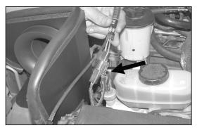
28. Reconnect the secondary mass air electrical connection as shown.
