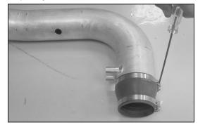
18. Install the provided silicone step hose and hose clamps onto the K&N<sup>®</sup> intake tube and tighten as shown.
