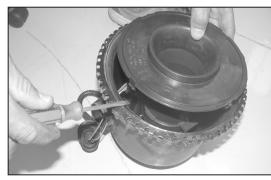
11. Using a flat blade screwdriver release the housing cover and pull up as shown.
