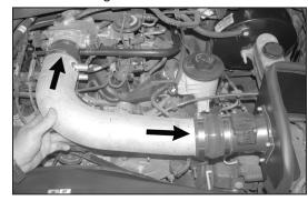
21. Slide the K&N<sup>®</sup> intake tube into the silicone hump hose, then, slide the silicone step hose onto the throttle body as shown.
