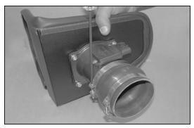
16. Install the silicone hump hose and hose clamps onto the mass air sensor and tighten as shown.
