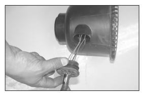
10. Disassemble the air cleaner assembly, then, pull the plastic wire cover and rubber boot back on the mass air electrical connection as shown.
