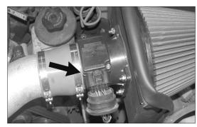
26. Reconnect the primary mass air sensor electrical connection as shown.
