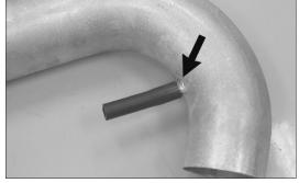
20. Install the provided silicone hose onto the vent on the K&N® intake tube as shown.
