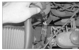
25. Reconnect the secondary mass air electrical connection as shown.
