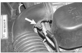
3. Disconnect the crank case vent hose from the stock intake.
