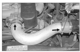
21. Slide the tube into the silicone hose on the mass air sensor, then, slide the other end into the silicone hose on the throttle body, adjust everything for best fit and clearance, then, tighten all hose clamps and hardware as shown.
