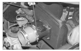
15. Install the silicone step hose and hose clamps onto the mass air sensor and tighten as shown.
