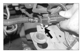
6. Remove the mass air wire harness from the air cleaner support bracket, which is located below the air cleaner assembly.
