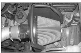
24. Install the K&N® air fitler and secure with the provided hose clamp as shown.
