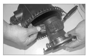
10. Pull the mass air sensor out of the housing and disconnect the mass air sensor electrical connection as shown.
