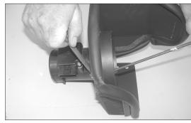
13. Assemble the provided mass air adapter, gaskets, heat shield and the stock mass air sensor using the provided hardware as shown.
