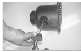
8. Disassemble the air cleaner assembly, then, pull the plastic wire cover, and the rubber boot back on the mass air electrical connection as shown.
