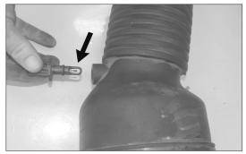
17. Remove the air temperature sensor from the stock intake tube as shown.
