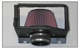
14. Install the provided silicone hose (08699) onto the filter adapter as shown. Secure with the provided hose clamp.
