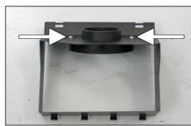
9. Install the K&N $^{\!(\!0\!)}$  filter adapter into the heat shield as shown. Secure with the provided hardware.
