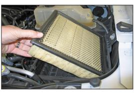
7. Remove the air filter from the lower airbox.
