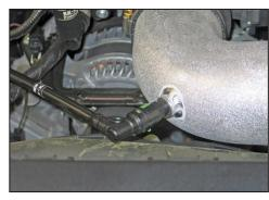
21. Rotate the crankcase vent coupler so it lines up with the fitting installed into the K&N<sup>®</sup> intake tube; connect the coupler to the fitting.
