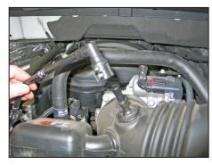
3. Release the green locking tab and then disconnect the crankcase vent line from the intake tube as shown.
