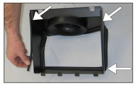
12. Install the two 9-1/2" lengths of small edge trim onto the heat shield as shown.
