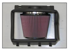
13. Install the  $K\&N^{\textcircled{R}}$  air filter onto the filter adapter and secure with the provided hose clamp.
