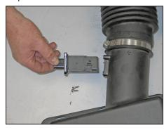
17. Remove the two screws securing the mass air sensor to the factory airbox, and then remove the mass air sensor.
