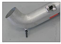
19. Install the provided crankcase vent fitting into the  $K\&N^{\circledR}$  intake tube as shown.
