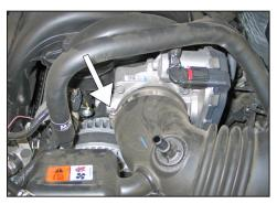
4. Loosen the hose clamp that secures the intake tube to the throttle body.
