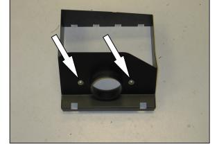
11. Install the K&N<sup>®</sup> filter adapter into the heat shield as shown and secure with the provided hardware.
