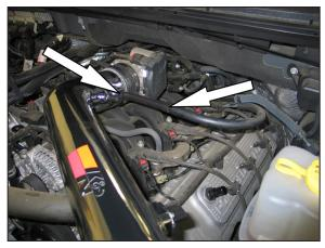
23. Install the hose mender into the provided EVAP hose, then install the hose mender into the factory EVAP hose and attach the open end onto the vent fitting installed into the K&N<sup>®</sup> intake tube.
