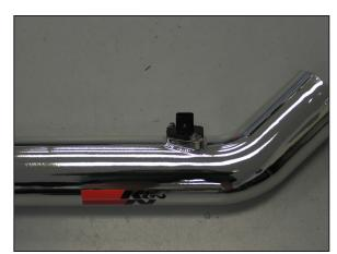
20. Install the mass air sensor into the  $K\&N^{\circledast}$  intake tube as shown and secure with the provided
