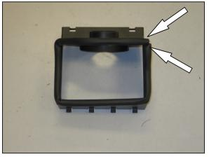
14. Install the provided "Top bulb" edge trim onto the top off the heat shield as shown. **NOTE: Some trimming of the edge trim will be necessary**.
