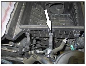
16. Remove the middle upper air box retaining clip from the lower air box.
