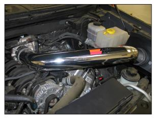
22. Install K&N<sup>®</sup> intake tube into the silicone hose at the filter adapter and then into the hose at the throttle body, adjust the tube for proper fit and then secure with the provided hose clamps.
