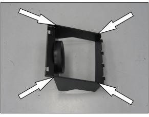
13. Install the cut edge trim onto the bottom of the heat shield as shown.
