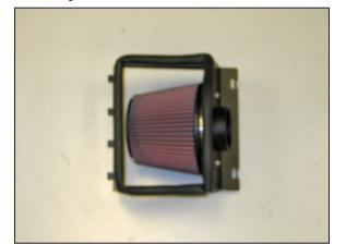
15. Install the K&N<sup>®</sup> air filter onto the filter adapter and secure with the provided hose clamp. **NOTE: Drycharger<sup>®</sup> air filter wrap; part # RC-5173DK is available to purchase separately.**
