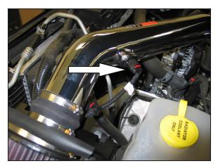
25. Connect the provided mass air sensor extension harness into the factory harness and then connect to the mass air sensor, secure the wiring harness with the provided tie wrap.
