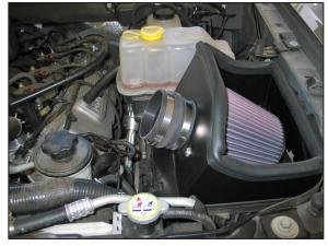
18. Install the provided silicone hump hose (08699) onto the filter adapter and secure with the provided hose clamps.
