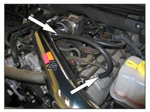
24. Install the provided crank case vent hose onto the valve cover port and then onto the vent installed into the K&N<sup>®</sup> intake tube as shown.
