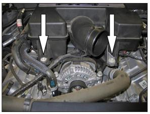
6. Remove the two bolts securing the intake plenum onto the intake manifold.
