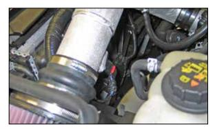
22. Reconnect the mass air sensor electrical connection.
