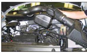
6. Release the three clips securing the upper air box housing to the lower housing and then remove the intake tube/upper airbox and air filter from the vehicle.
