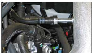
20. Connect the crankcase vent hose to the quick disconnect fitting on the K&N® intake tube. NOTE: It is necessary to rotate the plastic crank case vent tube on the plastic connector that attaches to the valve cover approximately  $\frac{1}{4}$  turn counter clockwise for the tube to align with the fitting on the K&N® intake tube.
