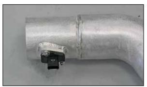
18. Install the mass air sensor into the K&N<sup>®</sup> intake tube and secure with the provided hardware.
