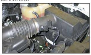
2. Release the red locking tab and then disconnect the mass air sensor electrical connection.
