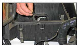
12. Remove the center airbox retaining clip.
