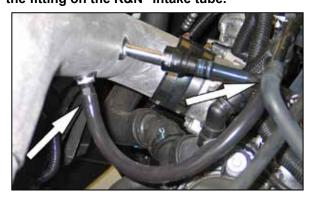
21. Install the provided silicone hose onto the 3/8" hose fitting installed in the K&N® intake tube; attach the open end to the EVAP check valve.
