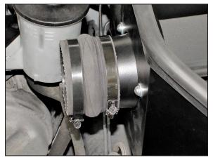
17. Install the provided hump hose (084057) onto the filter adapter and secure with the provided hose clamp.
