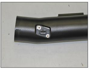
19. Install the mass air sensor into the K&N $^{\odot}$  intake tube and secure with the provided hardware.
