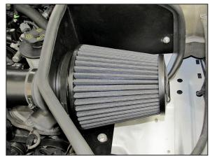
23. Install the K&N® air filter onto the filter adapter
