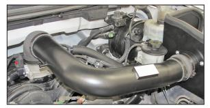
20. Install the K&N<sup>®</sup> intake tube into the 90° elbow hose and then into the hump hose, align for best fit and then secure with the provided hose clamp. **NOTE: On vehicles equipped a Brake Booster/ EVAP vent line, it will be necessary to align the vent line to the tube and mark the tube to be drilled. Remove the tube and drill a 5/8"id hole in the marked location and install the provided grommet, be sure to remove any burrs and shavings.**
