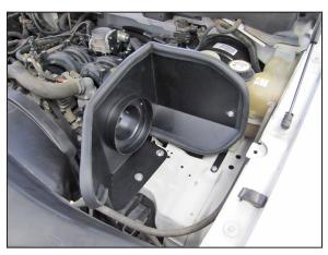
15. Set the heat shield onto the air box mounting plate so the inserts go into the mounting grommet holes. Secure the heat shield with the insert bolts and with the bracket to the inner fender with the provided hardware.
