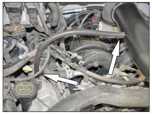
22. Install the provided crank case vent hose onto the vent port on the K&N<sup>®</sup> intake tube and then onto the vent on the valve cover.
