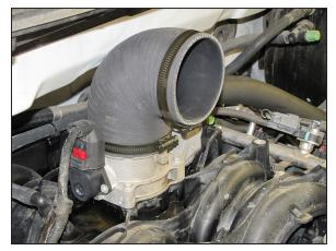
16. Install the provided 90° hose onto the throttle body and secure with the provided hose clamp.
