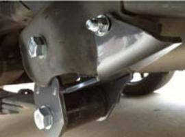
12. Install the Maxtrac shock absorber(s) in the stock location.
