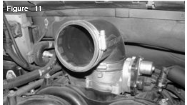
Take the 3 1/2" 90 degree elbow and two 56 clamps and insert short end of elbow over the throttle body.
