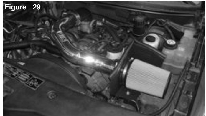
Figure 29 Congratulations! You have just completed the installation of this Power-Flow intake system. Periodically, check the fitment of the intake track and Power-box in order to avoid damage to the intake system that could void the warranty.
