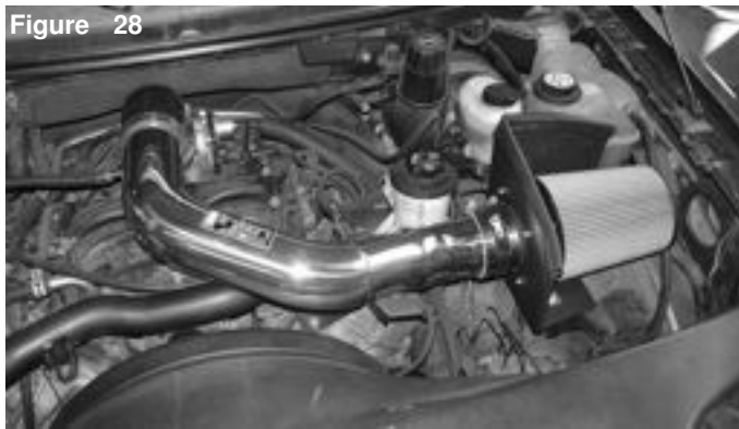
Figure 28 Check for clearance and position for the best possible fit. Re-tighten if necessary.
