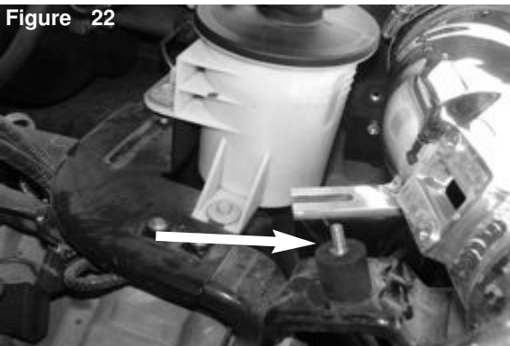
Figure 22 Position the bracket to the vibra mount from step 12.
