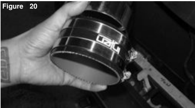
Figure 20 Install the straight hose with clamps to the end of the intake tube.
