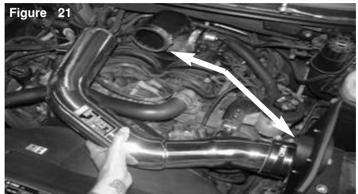
Figure 21 Install the intake tube and position to the throttle body and heat shield.
