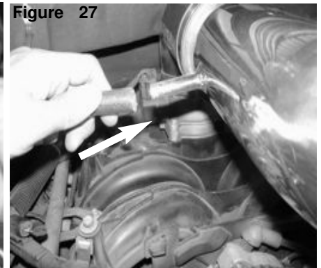
Figure 27 Attach the 10mm hose to the fitting on the intake tube.
