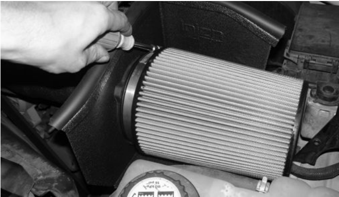
Install the air filter and tighten using 8mm nut driver. re-install the engine cover.
