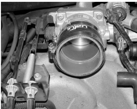
Press the 3" straight hose over the throttle body and use two clamps. Tighten the clamp on the throttle body side for now.
