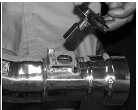
Insert the MAF sensor in into the machined MAF sensor adapter welded to the tuned intake.
