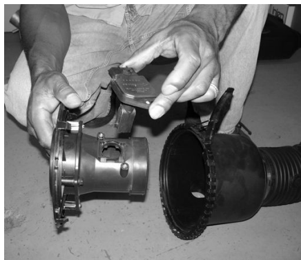
Using the T-20 torx bit in this kit remove the screws holding the MAF sensor to the plastic housing.
