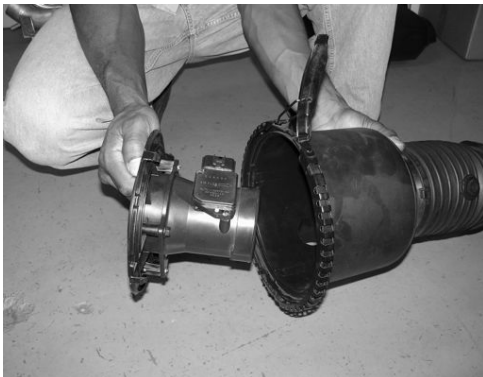
Remove the MAF sensor housing from the air intake box as shown above.
