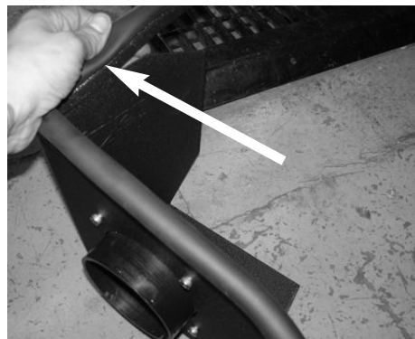
Attach the trim seal to the top of the heat shield.
