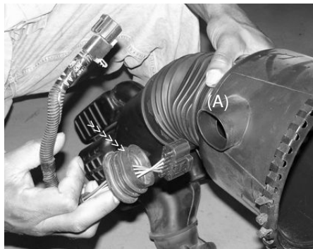
Remove plug from the air intake box (A) and remove the entire harness assembly in one piece.
