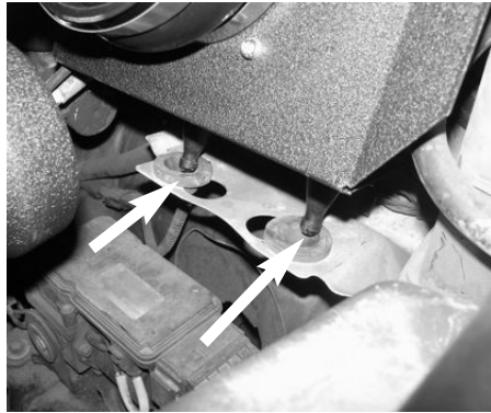
Secure the stand off studs and make sure that they are seated completely.
