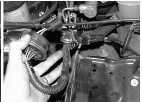
Reconnect the harness assembly to the female end of the main harness.
