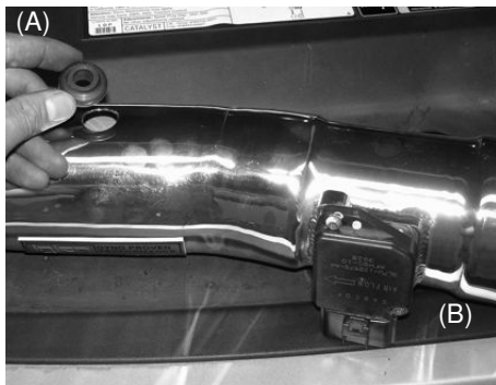
Insert the 1525 sensor grommet into the pre-drilled hole until the grommet groove is flush to the hole Inner diameter (A). Use the stock screws to fasten the MAF sensor to the machined adapter (B).
