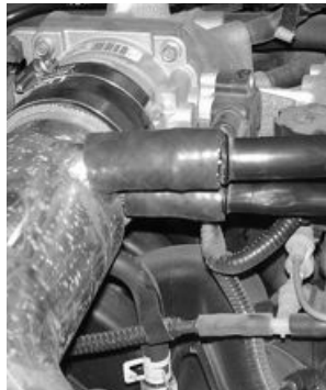
Cut the 22" long 17mm hose to 2-1/2" length if vehicle requires shorter hose length. Press the 2 1/2" long 17mm hose over the 3/4" port on intake (A). Insert the larger hard pipe into the the 17mm hose as shown above (B).
