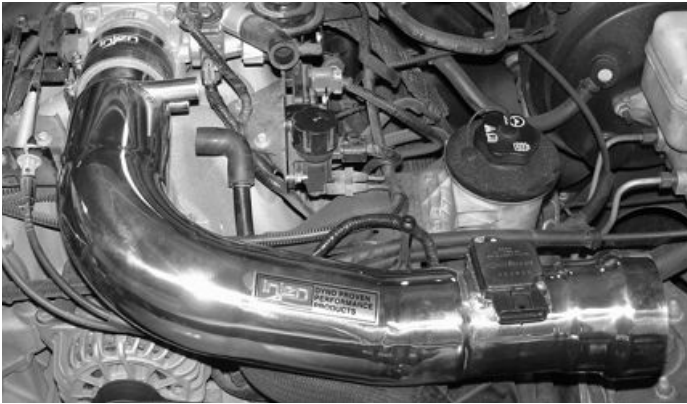
Take the Tuned intake and press the 3" side into the hose on the throttle body. Do not over tighten the clamp on the hose until the installation is complete.
