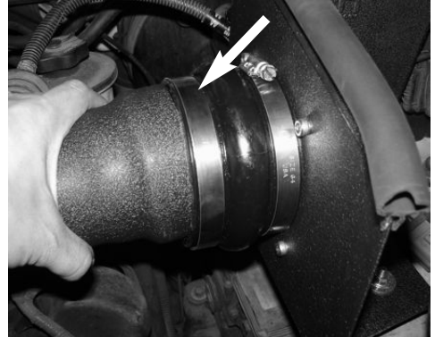
Connect the the tube and the hose, position for the best fit and tighten the clamps using 8mm nut driver.
