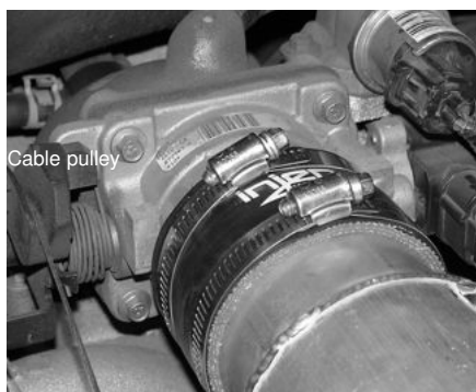
Place the clamping mechanisms right side up. This will keep the mechanism from hanging up to the cable pulley which could cause damage to yourself and others.
