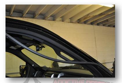
3. Carefully align top of mounts to top of the rivet located inside the door jamb, under the weatherstrip. Do this for both sides of the truck.
