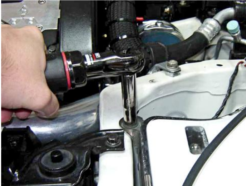
A second example of loosening headlamp assembly anchor bolts.
