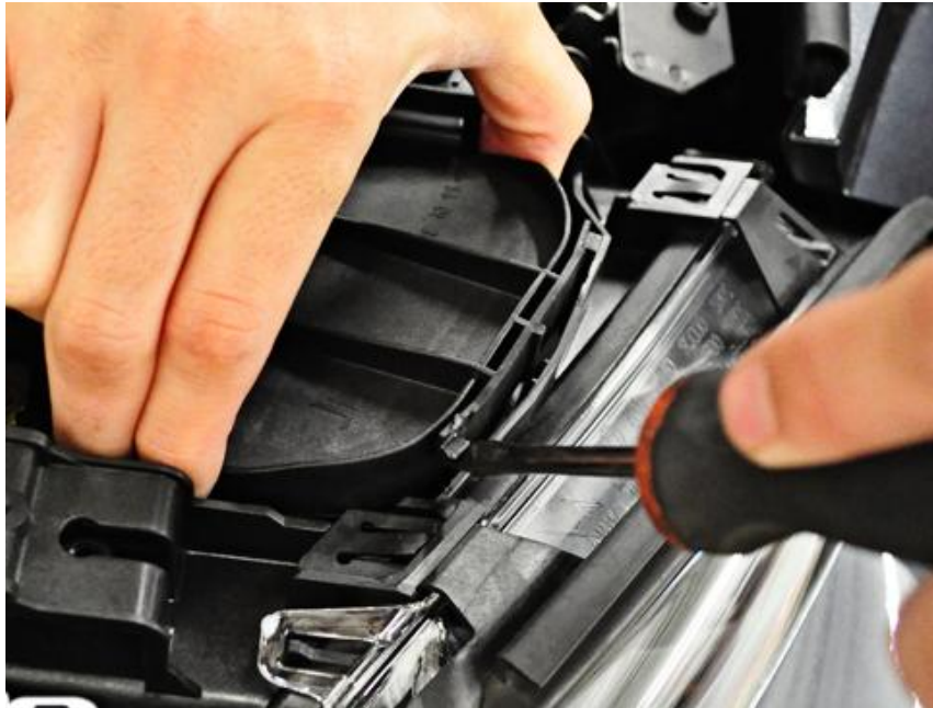
An example of hold-down clips that must be released before a headlamp assembly can be removed.
