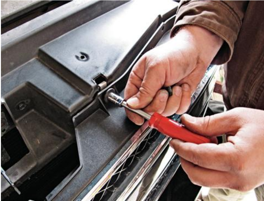
Removal of front grille sections to access headlamp anchor points is required on many vehicles.
