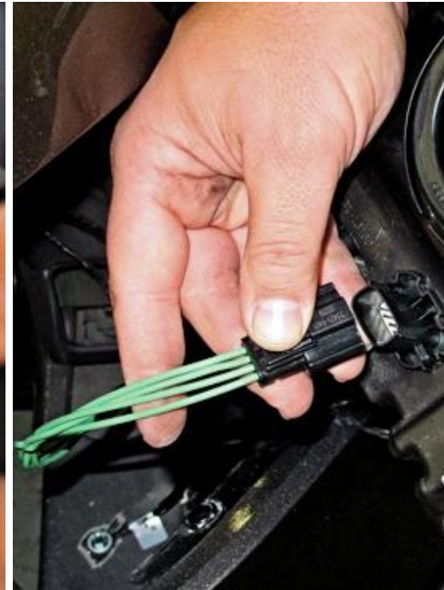
After all applicable hold-down bolts and clips have been removed, headlamp assemblies can be gently slid away from the vehicle.
