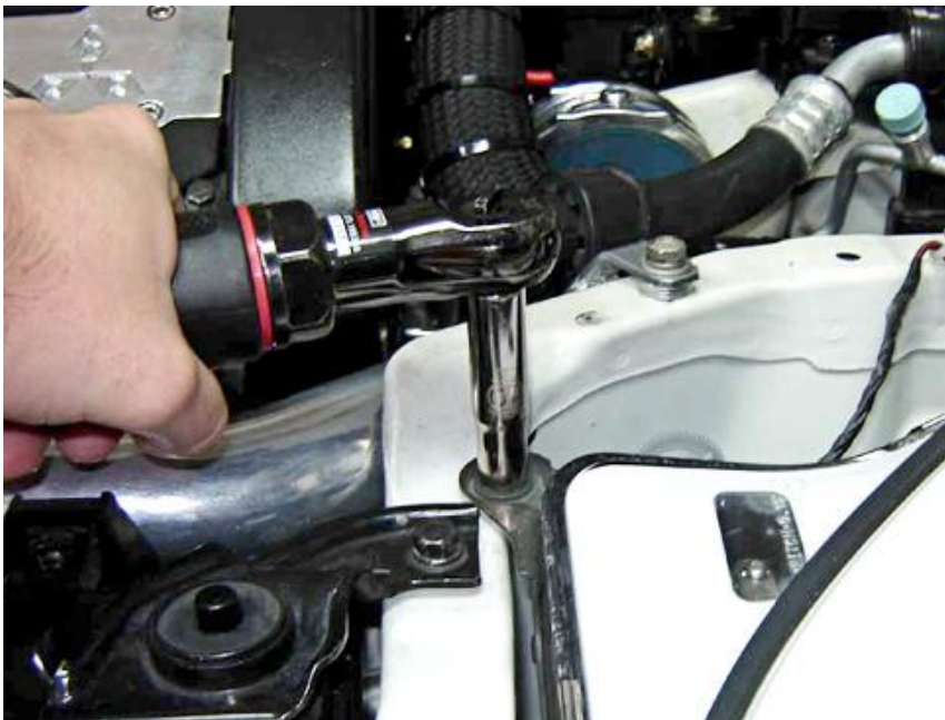
A second example of loosening headlamp assembly anchor bolts.
