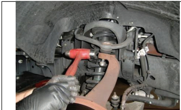
Strike with hammer to disconnect ball joint from spindle
