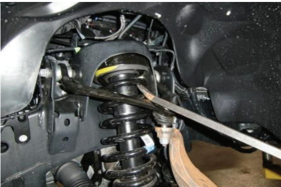
Use jack to raise suspension and reconnect upper ball joint
