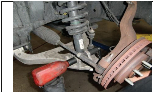
Remove lower strut mounting hardware
