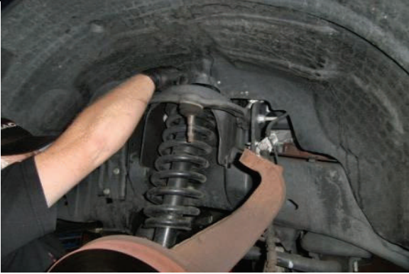
Remove strut upper mounting hardware & remove assembly
