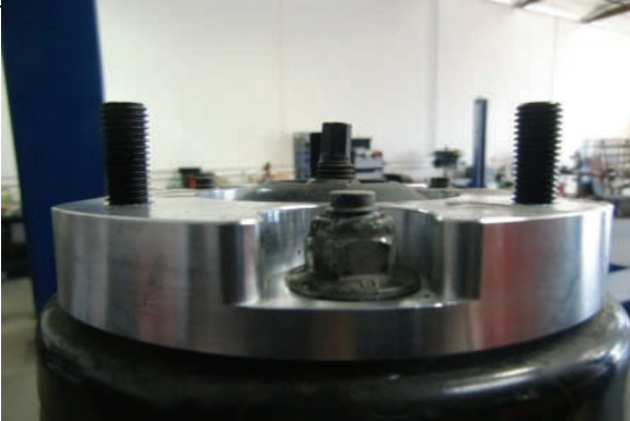
Bolt spacer to top of strut with OE hardware
