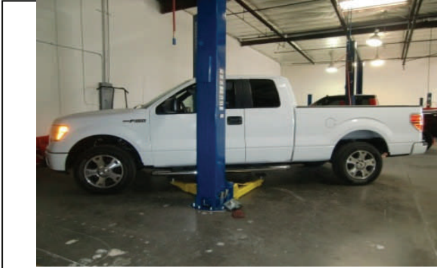
Measure vehicle on level surface and raise by frame
