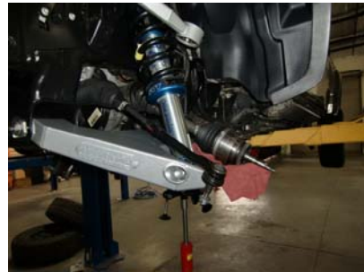
18. Install the lower shock into the lower control arm.
