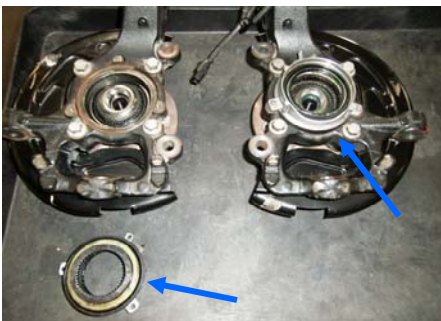
19. Remove the CV joint seal from both of the spindles.
