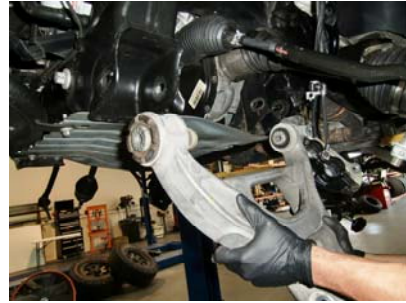
14. Unbolt and remove the lower control arm.
