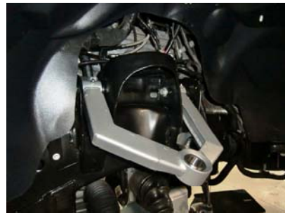
16. Install the ReadyLIFT® upper control arm.
