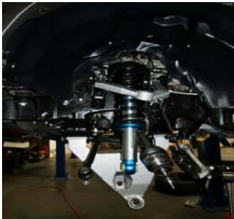
17. Re-install the shock at the top.
