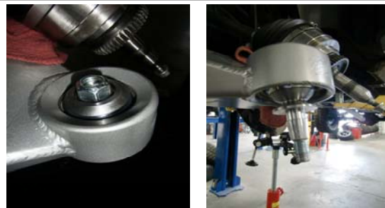
20. Install the misalignment spacers into the LCA uniball. Install the pin with a washer and c-lock nut hand tightened
