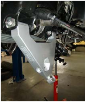
15. Install the ReadyLIFT® lower control arm.
