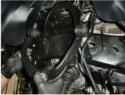
13. Unbolt and remove the upper control arm.
