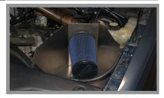
Install the BBK filter shield on the driver side inner fender. Use supplied bolts and washers to mount the shield.
