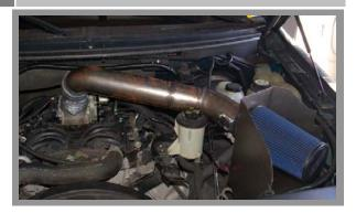
Install the chrome inlet tube into the hole in the filter shield then on to the connector on the throttle body. Rotate the inlet tube for the best position and tighten the clamps at the blue connector. Install the filter on to the end of the inlet tube and tighten the clamp.
