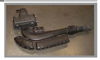
Remove the four retaining bolts for the stock air intake at the intake manifold. Remove the bolt just forward of the power steering reservoir that holds the inlet tube. Remove the assembly from the vehicle.
