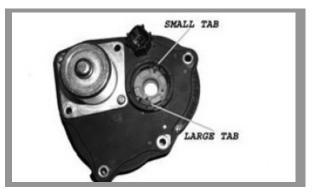
Using needled nose pliers, rotate the plastic spring cap <u>COUNTER-CLOCKWISE</u>
