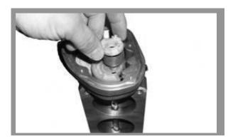
Place the plastic capped spring over the end of the throttle shaft of the BBK Throttle Body and line the pig tail hook on the spring up with the catch slot in the gear.
