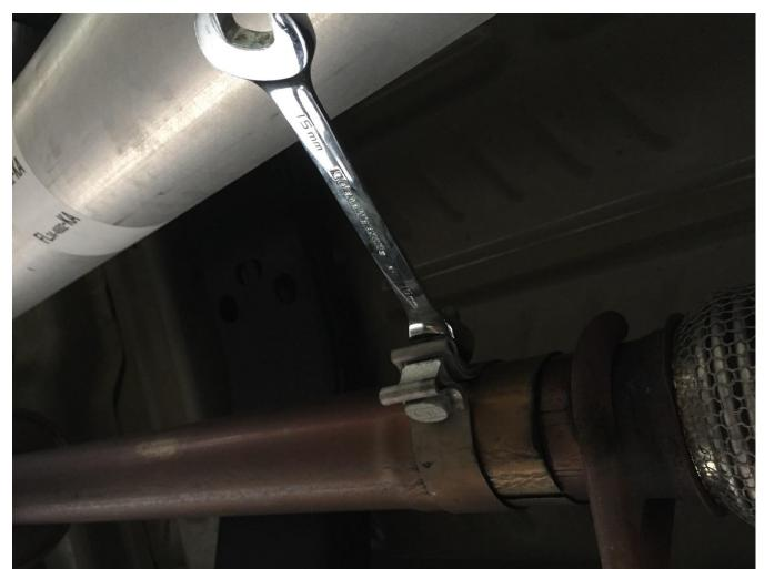
3. Using a 15mm Wrench start to loosen the bolt connecting band clamp to the flex pipe. You do not need to completely remove the nut, once loose the pipe will move freely. This will allow the locking design to rotate out allowing for separation.
