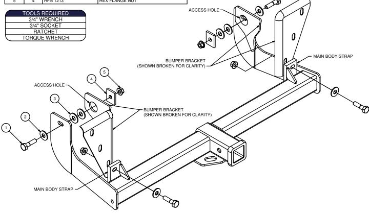
HITCH WEIGHT:  $\underline{35}$  LBS. INSTALL TIME:  $\underline{15}$  MINUTES INSTALL NOTES:
