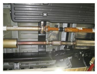
**Step 2.** To begin, fasten the Inlet Pipe Assembly to the catalytic converter using the OEM clamp assembly and by fitting the welded hanger into the OEM rubber insulator (Leave all clamps and fasteners loose for final adjustment of the complete system.) Install the Muffler to the Inlet Pipe Assembly using the supplied 3.00" clamp and fitting the hanger. Next install the Tailpipe Extension Assembly to the Muffler in the similar fashion using the supplied 2.50" clamps.
