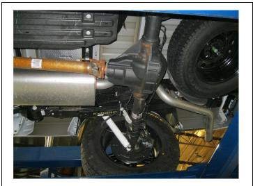
**Step 1.** To remove the OEM exhaust system, you will to need to cut the pipe behind the muffler before it goes over the axle. You can then disengage the welded hangers from the OEM rubber insulators and remove the tailpipe. Unfasten the clamp attaching the OEM muffler inlet to the OEM catalytic converter. Do not damage or discard the OEM fasteners or rubber insulators, as they will be reused to mount the new system. Disengage the muffler hangers and remove the OEM exhaust from the vehicle
