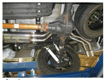
**Step 3.** Finish by installing the Tail Pipe Assembly to the Tail Pipe Extension Assembly using the supplied 2.50" clamps, fitting the welded hanger into rubber insulator.
