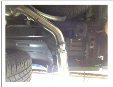
**Step 5.** Finish installing the components by sliding the Tailpipe Assembly onto the Over Axle Pipe and fastening with a supplied 3.00" Clamp. Fit the hanger into the rubber insulator.
