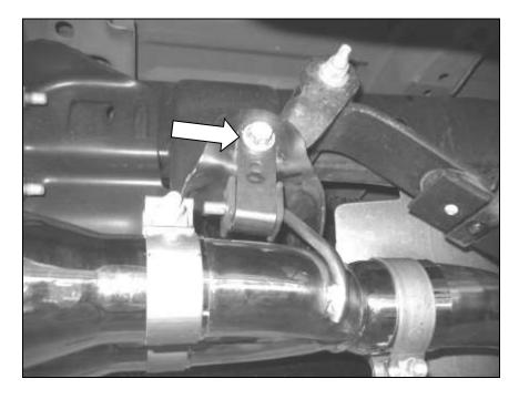
15. With the full system now hanging in the truck, make sure all of the hangers are fully seated and there are no clearance issues with vehicle parts contacting the exhaust system.
