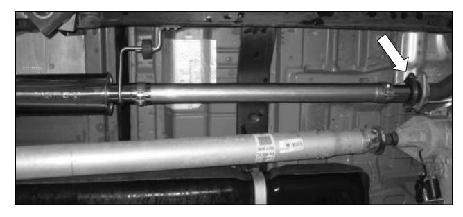
11. Install one (1) 2.5" clamp (R12060014) onto each of the exhaust tips and slide the tips onto the ends of the Y-pipe. Position the clamps on the pipe joints and loosely secure the clamps.
