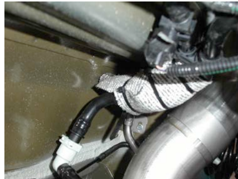
Wrapped EVAC Tube (picture #2)
