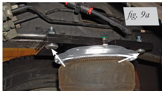
Left hand assembly (driver side) attached with carriage bolts (R), flat washers (M) and nylon lock nuts (U). Torque to 31ft. lbs.
