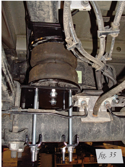
Left side (driver): rear view of installation.
