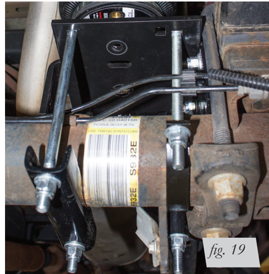
Right side (passenger) rearward axle view of finished installation torqued to 10ft. lbs.
