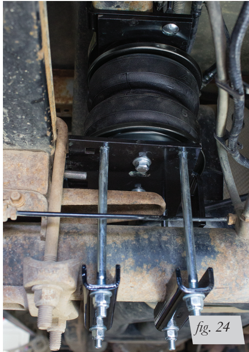
Left side (driver): rear view of installation.
