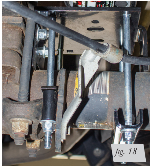
Right side (passenger) forward axle view of finished installation torqued to 10ft. lbs.
