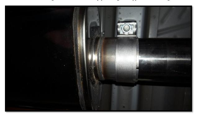
**Step 6**: Once you position your exhaust in the exact location that you like, start tightening all your bolts and clamps starting at the front of the exhaust with the flange making sure your evenly tighten this. Then tighten the TORCA clamp where the muffler assembly and the inlet pipe meets together. Lastly you will need to tighten the two bolts on the outside of the frame holding the tailpipes up.
