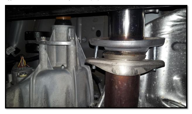
**Step 2**: Locate and remove the second rubber exhaust hanger and bushing on the inside of the trucks frame by remove the two 10mm bolts shown in the picture. If you have the 5.0 engine you will need to leave this in place.
