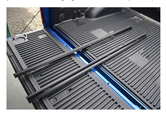
2. Grab one of the Side Rails and position the top edge of the rail 1/8 in. above the top edge of the F-150 bed rail.
