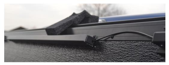
12. Once the cover is in the open position, go back and tighten the clamps that are attaching your Side Rails to the truck Bed. Do not over tighten the clamps, a torque wrench is not needed, if you want to use one, only tighten the bolts to approximate 75 inch lbs.
