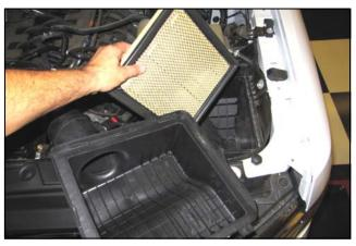
**3.** If installing the Airaid Jr. Kit, unfasten the three clips on the left side of the factory airbox, and remove the upper half of the factory airbox. Remove the factory air filter element.
