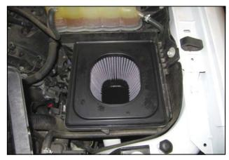
4. Install The Airaid Premium Filter (#1) into the air-
