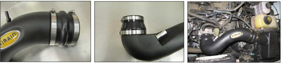
**7.** Install the hump hose (#3) and two #60 hose clamps (#9) onto the Intake Tube as shown. Leave the hose Clamps loose for now.
