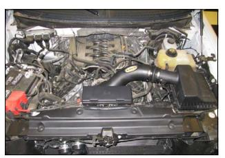
11. Double check your work! Make sure there is no foreign material in the intake path. Make sure all clamps, hoses, bolts, and screws are tight. Double check the hood clearance! **Reconnect the negative battery cable!**
