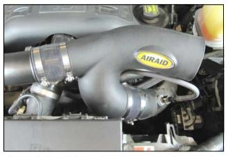
**6.** Install the Airaid Intake Tube onto the factory turbo plumbing and tighten the Clamps. Reconnect the vacuum line if so equipped
