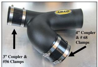
**5.** Slide the Couplers and Clamps onto the Intake tube as shown. Apply the Airaid Bubble Decal onto the Intake Tube as shown.
