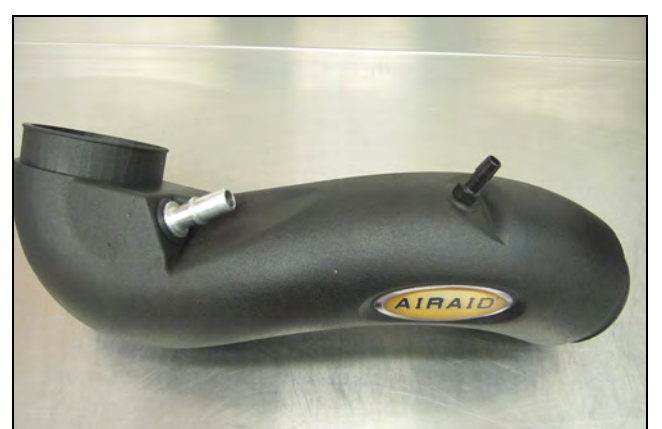
6. A.) Install the 3/8 " Barbed Fitting (#5) into the threaded holt in the Intake Tube. B.) Insert the 5/8" Grommet (#7) into the Intake tube as shown. Complete the tube assembly by inserting the 5/8 PCV Fitting (#6) into the Grommet.
