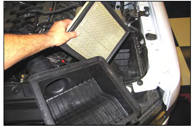
3. Unfasten the three clips on the left side of the factory airbox, and remove the upper half of the factory airbox. Remove the factory air filter element.
