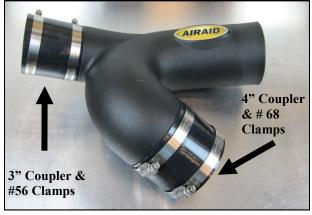
**5.** Slide the Couplers and Clamps onto the Intake tube
