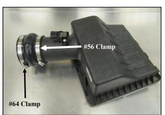
**7.** Slide the Hump Hose and the two remaining Clamps onto the OEM air box lid as shown.
