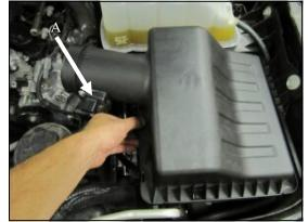
2. A.) Disconnect the Mass Air Flow (MAF) Sensor.
