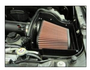
**9.** Install the Airaid Premium Filter (#1) to the mounting flange inside the quick fit assembly. Complete the installation by attaching the Weather Strip (#5) to the top of the panels as shown.
