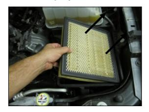
**3.** Remove the factory air filter from the lower half of the airbox.
