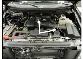
**1. Disconnect the negative battery cable!**Loosen the two intake clamps and remove the Factory intake tube.
