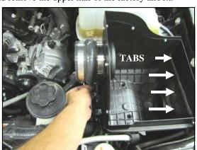
**5. A.**) Install the Silicone Hump Hose (#7) and two #64 Hose Clamps(#14) onto the Quick Fit assembly. Leave the clamps loose for now.
