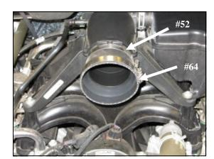
**6.** Install the Silicone Coupler (#6), one #64 Hose Clamp(#14), and the #52 Hose clamp (#13) onto the engine air inlet. Leave the clamps loose for now.
