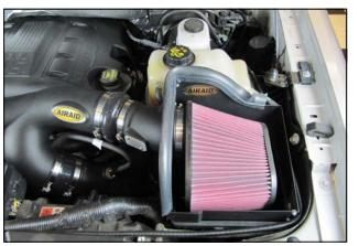
14. Install the Airaid Premium Filter onto the Sensor Tube and tighten the clamp.
