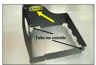
**6.** Assemble the Front and Rear Panels as shown with the tabs on the outside of the assembly. Use the four 6-32 Phillips Head Screws, #6 Flat Washers, and #6 Kep Nuts to secure the assembly. Complete the Panel assembly by applying the Airaid Foil decal.
