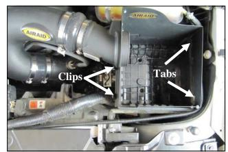
12. Install the Tube and Panel assembly onto the Airaid Intake Tube first, then insert the Panel tabs into the factory air box slots. Adjust the assembly until the OEM air box clips can positively engage the Panels and lock.
