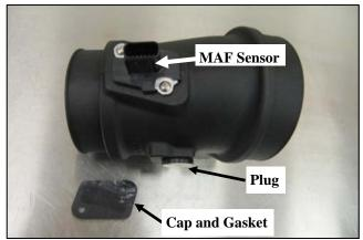
9. If your vehicles intake utilizes a Mass Airflow, or MAF sensor: Transfer the sensor into the Airaid Sensor Tube as shown and secure using the two 1/2" Button Head Screws. Complete the Tube assembly by inserting the MAP Plug. Discard the Meter Cap and Gasket. They will not be used.
