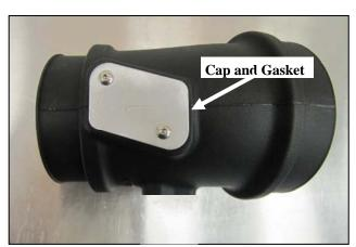
**7. If your vehicles intake utilizes a MAP sensor**: Install the Meter Cap and Gasket onto the Airaid Sensor-Tube as shown, using the two 8-32 1/2" Button Head Screws.
