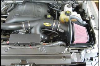
15. Double check your work. Make sure there is no foreign material in the intake path. Make sure all clamps, hoses, bolts, and screws are tight. Double check the hood clearance.
