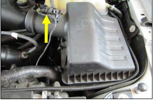
**2.** Disconnect the wiring harness from air sensor in the air box lid. Unclip the air box lid and remove it and the factory air filter from the vehicle. The lower half of the factory air box is to remain in the vehicle.
