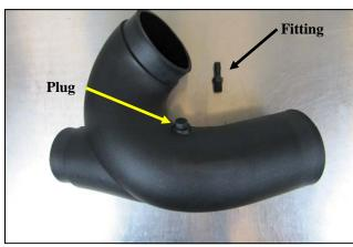
**3.** On 2011 models with the vacuum line in the intake, install the 1/4" Barbed Fitting. The Plug will not be used. On 2012-2014, Install the 1/4" Plug into the Airaid Intake Tube as shown.
