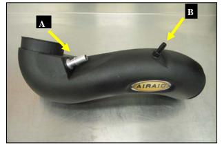
9. A.) Insert the 5/8" Grommet into the Intake tube as shown. Complete the tube assembly by inserting the 5/8 PCV Fitting into the Grommet. **B.**) Install the 3/8 "Hose Fitting into the threaded holt in the Intake Tube. Complete the Tube assembly
