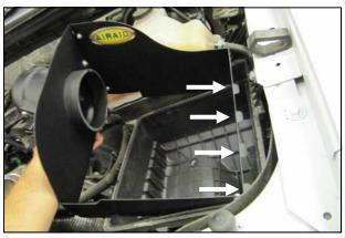
8. Install the assembly onto the lower half of the factory airbox. Slide the metal tabs into the airbox slots, and fasten the 3 airbox clips
