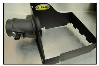
**6.** Transfer the **MAF** sensor into the Airaid Intake Tube and secure using two 8-32 x 1/2" button head screws. **Do Not Use The Factory Torx Head Screws.**
