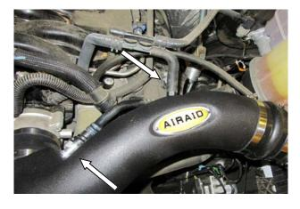
14. Reconnect the breather lines to the Airaid Intake Tube.
