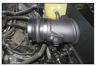
**12.** Install the hump hose and two hose clamps onto the filter Air Meter Tube as shown. Leave the two hose clamps loose for now
