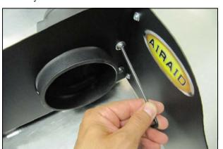
7. Install the Air Meter Tube onto the Panel Assembly and secure using the two 1/4-20 Button Head Bolts, and 1/4" Flat Washers.
