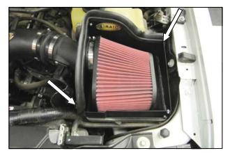
16. Install the Weather Strip onto the panel assembly with the contoured edge rolling away from the filter area. Start at the front of the vehicle and work your way back. Complete the installation by sliding the Airaid Premium Filter onto the Air Meter Tube and tightening the clamp.
