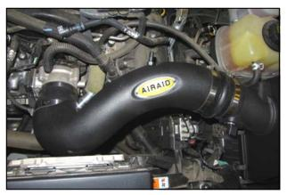
13. Install the Intake Tube onto the throttle body first, then into the Hump Hose. Tighten all of the hose clamps.
