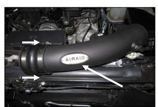
7. Install the Hump Hose (#5), and the clamps (#13) onto the Intake Tube. Slide the hump hose and clamps down the tube as far as they will go and leave the clamps loose for now. Apply the Airaid Bubble Decal to the Tube assembly as shown
