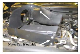
**4.** Assemble the two Quick Fit panels (#3 & #4) as shown using four 6-32 screws (#7) flat washers (#9) and kep nuts (#8). Apply the Airaid Foil Decal to the Panel assembly as shown.
