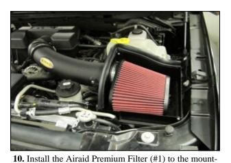
ing flange inside the quick fit assembly. For **SVT Raptor** vehicles: Complete the installation by attaching the Short Weather Strip (#6a) to the top of the panels as shown.
