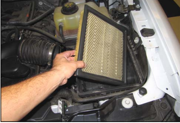
4. Remove the Factory air filter.
