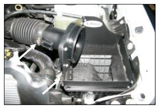
6. Install the Quick Fit Assembly onto the top of the factory airbox base sliding the four tabs on the panel into the slots on the base and then latching the three factory latches. Slide the factory intake tube over the **MAF** tube and tighten the factory hose clamp as about
