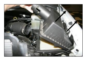
**2.** Remove the factory airbox lid from the vehicle by sliding the flexible tube off of the airbox lid neck, and then rotate the lid up and out of the base.
