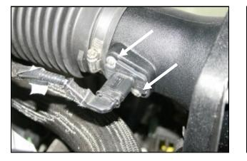
7. Reinstall the MAF sensor into the Airaid Adapter Tube using two 8-32 x 3/8" button head screws (#11). Do Not Use The Factory Screws !
