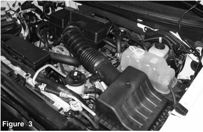
Figure 4 Loosen clamp on air box resonator using 8mm nut driver.
