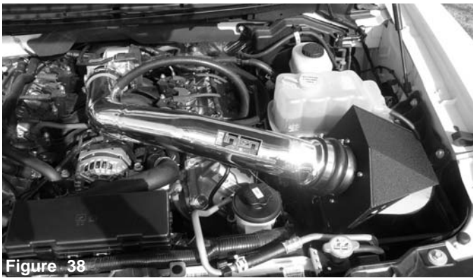
Figure 38 Check the entire system for the best possible fit. Once you have checked the entire system for leaks, rubbing or rattling, continue to tighten all nuts, bolts and clamps. Reconnect the negative battery terminal prior to starting the engine.
