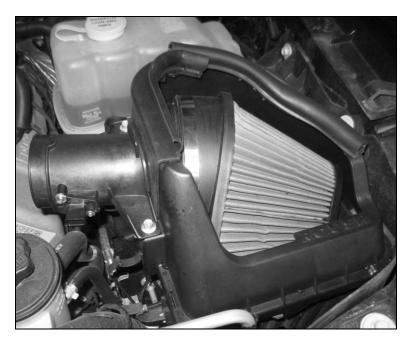
13. Connect the clean air tube to the new ROUSH air box lid assembly. Secure the clamps for the air box lid and tighten the clamp on the clean air tube to the MAF Tube.
