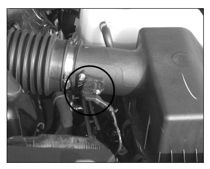
3. Loosen the hose clamp that connects the clean air tube to the airbox lid and disconnect the clean air tube at this joint. Note – Do not remove the clean air tube from the vehicle.
