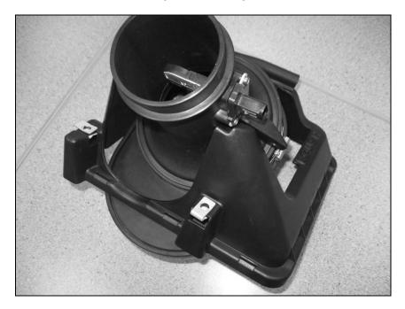
9. Install the EPDM close out seal (1111-9645) around the MAF Tube and clip into the edges of the upper air box tray.
