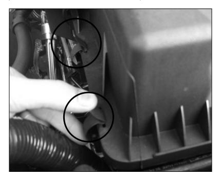
5. Transfer the MAF sensor and fasteners from the factory air box lid to the new ROUSH MAF tube (1111-12B579). Torque bolts to 1.8 - 2.2 Nm.
